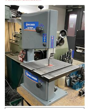
**Description:** Machine to cut out complex shapes and angles in smaller metal, plastic, or wood materials.
