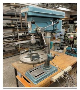
*Description:* On a fixed stand, drill accurate holes, countersinks and counterbores.
