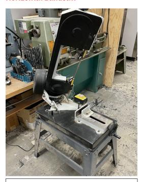
**Description:** A saw machine with a cutting arm brought down on the workpiece to cut through material. Typically used to cut down longer lengths of material.
