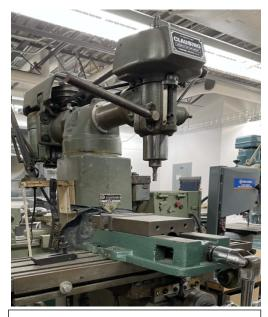
Description: Machine using rotary cutters to remove material along three axes. Can cut material, create slots, grooves, pockets, and other shapes from material. Accurate to within a thousandth of an inch.
