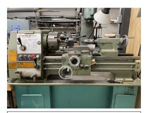
Description: A machine for shaping metal, wood, or other material by means of a spinning clamp. Turns the piece being worked on against changeable cutting tools for round cuts such as round grooves or sizing material to a precise diameter. Can be used for boring holes in round parts as well.
