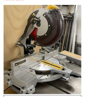
Description: Circular saw blade to cut through wood and some plastic material up to 8 inches wide. Can cut accurate angles from 0 to 90 degrees.
