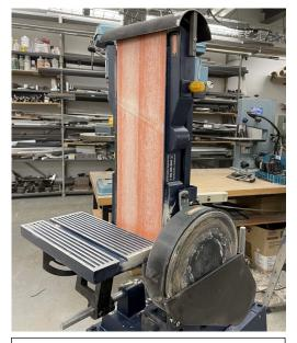
**Description:** A sander using a moving abrasive belt to smooth surfaces, flatten corners and remove thin layers of material.
